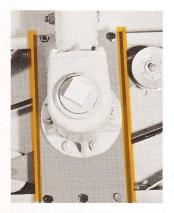
SPINDLES—they'll last as long as Methuselah anyway. But to be on the safe side, beef up the plate they mount on so they will stay put, rigid and in alignment.
